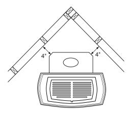
Figure 4 - Clearance for Corner Installation
